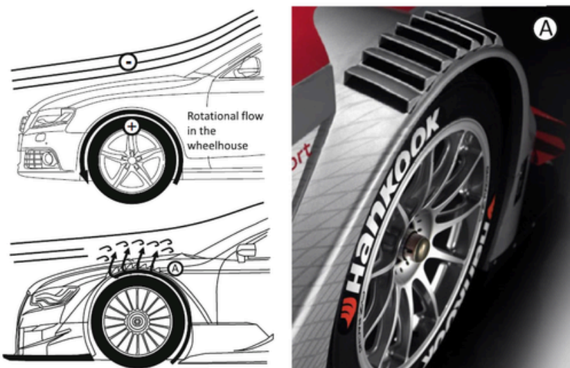
Fig. 6.99 Wheelhouse venting through Louvers. (Photo at right courtesy of © Audi AG 2018. All Rights Reserved)
