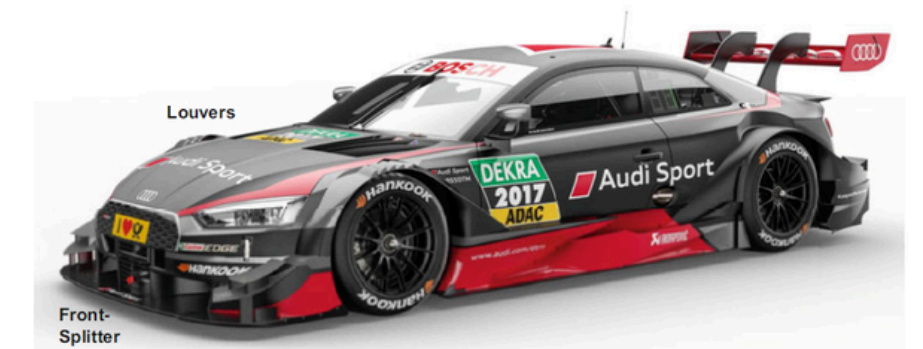
Fig. 6.96 Audi RS5 DTM with front splitter and louvers. (Courtesy © Audi AG 2018. All Rights Reserved)
